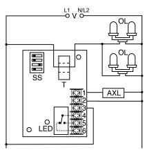
V = Voltage OL = Obstruction Lamps T = Toroid SS = Selector Switch AXL = Auxiliary Load/Alarm
