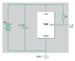
Note: It is strongly recommended that an external bypass capacitor be connected in-close-proximity to the device between the supply and ground pins to reduce noise. The recommended value for the external bypass capacitor is 0.1µF.
