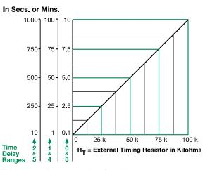
This chart applies to externally adjustable part numbers. The time delay is adjustable over the time delay range selected by varying the resistance across the  $\mathsf{R}_{\mathsf{T}}$  terminals; as the resistance increases the tie delay increases.
