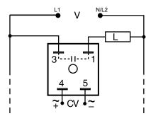
V = Voltage CV = Control Voltage L = Load
