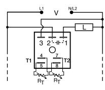
V = Voltage L = Load T1 = Delay-on-Make time
