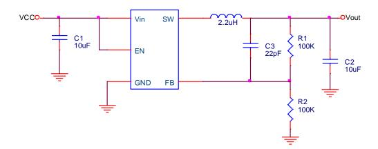
Adjustable Voltage Application Circuit
