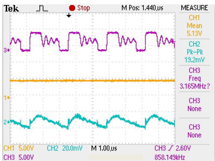
VIN=3.7V IOUT=50mA (CH1=VOUT CH2=VP-P CH3=SW)
