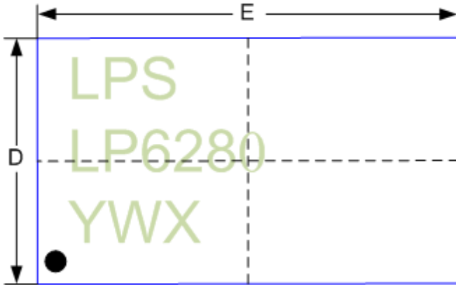
WLCSP-15-ball Package (1.4x2.3) pitch 0.4 (Unit: mm)
