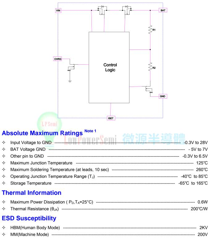
**Note 1.** Stresses beyond those listed under "Absolute Maximum Ratings" may cause permanent damage to the device. These are stress ratings only, and functional operation of the device at these or any other conditions beyond those indicated in the operational sections of the specifications is not implied. Exposure to absolute maximum rating conditions for extended periods may affect device reliability.
