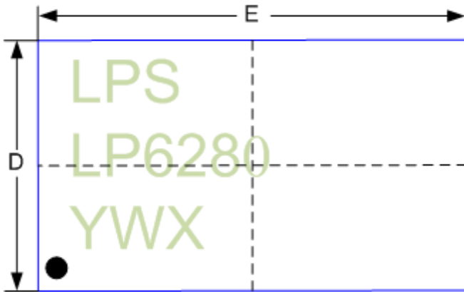
WLCSP-15-ball Package (1.4x2.3) pitch 0.4 (Unit: mm)
