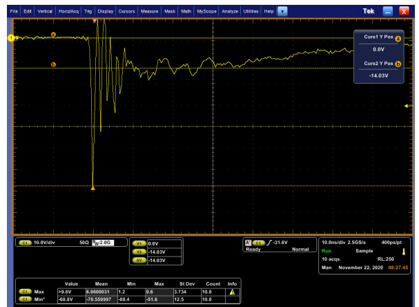
Fig 6. Negative 8kV contact per IEC61000-4-2
