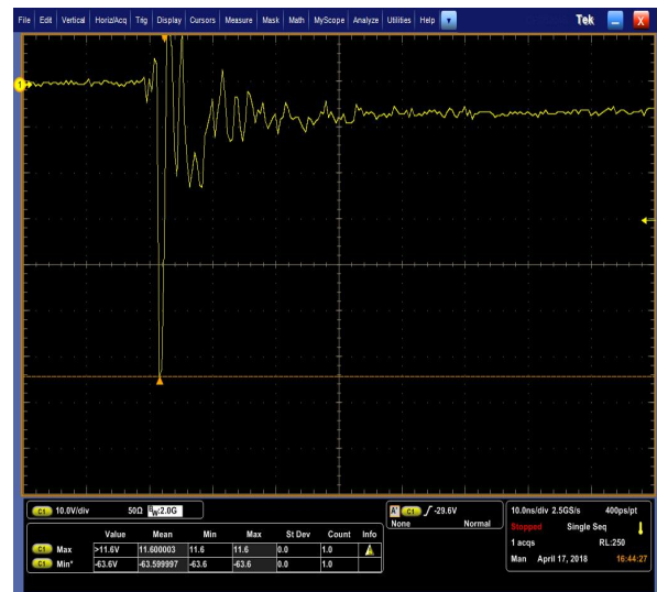
Fig2. ESD Clamping Voltage Screenshot Negative 8 kV Contact per IEC61000-4-2
