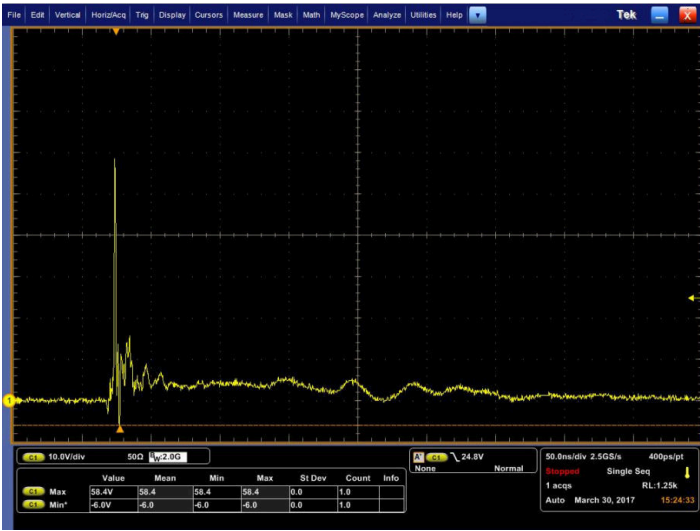
Fig4. ESD Clamping Voltage Screenshot Positive 8 kV Contact per IEC61000-4-2
