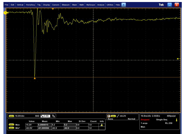
Fig4.Negative 8 kV Contact per IEC61000.4.2
