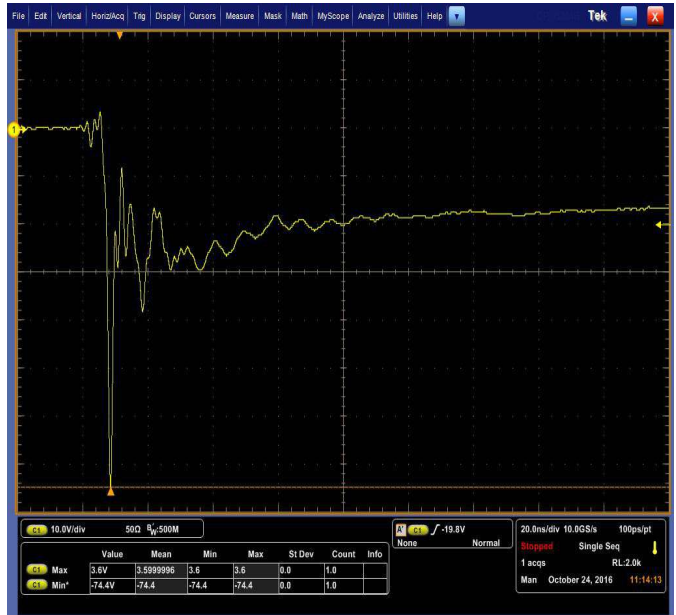
Fig 2. Negative 8kV contact per IEC 61000-4-2-LESD11D12CT5G
