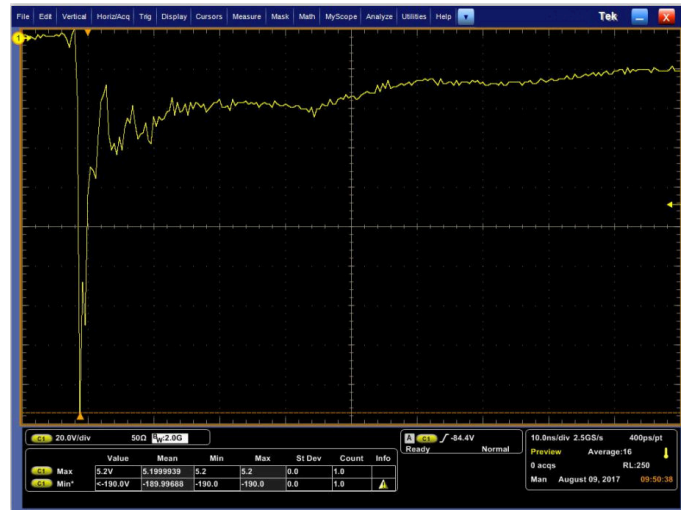
Fig4. ESD Clamping Voltage Screenshot Negative 8 kV Contact per IEC61000-4-2
