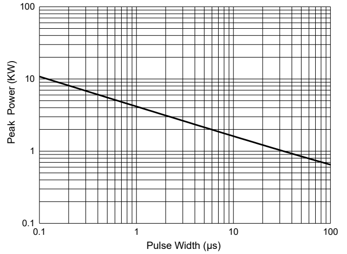
Fig. 2 - Peak Pulse Power Rating Curve
