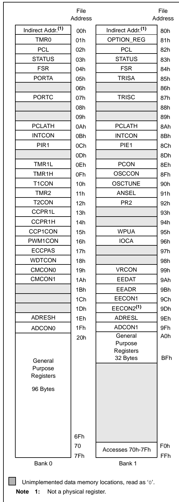
FIGURE 2-2: DATA MEMORY MAP OF THE PIC16F684
