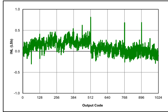
FIGURE 31-80: ADC 10-bit Mode, Single-Ended INL, V_{DD} = 3.0V , T_{AD} = 4\ \mu S , 25^\circ C .
