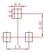
Note: 1.Controlling dimension:in millimeters. 2.General tolerance:± 0.05mm. 3.The pad layout is for reference purposes only.
