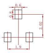
Note: 1.Controlling dimension:in millimeters. 2.General tolerance:± 0.05mm. 3.The pad layout is for reference purposes only.
