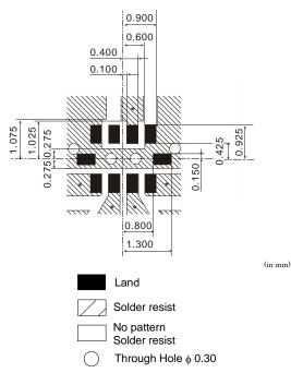
$\%\square$  Line width to be designed to match 50  $\Omega\,$  characteristic impedance, depending on PCB material and thickness.
