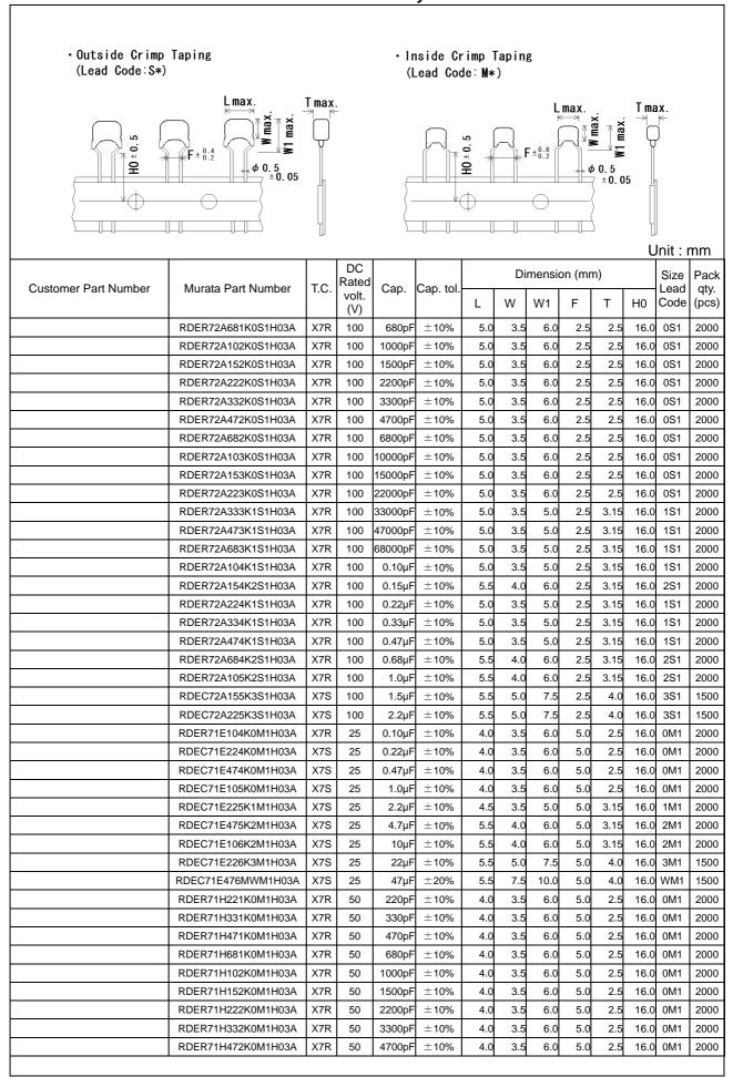
Inside Crimp Taping (Lead Code: M\*)
