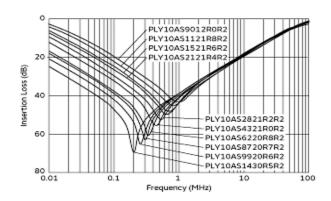
Common Mode Insertion Loss (Typ.)
