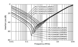
Common Mode Insertion Loss (Typ.)
