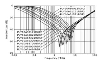
Differential Mode Insertion Loss (Typ.)
