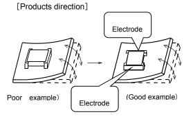
Products shall be located in the sideways direction (Length:a<b) to the mechanical stress.
