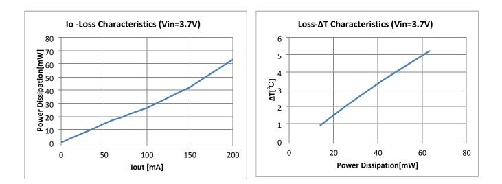
The output current of the device may need to be de-rated if it is operated in a high ambient temperature or in a continuous power delivering application. The amount of current de-rating is highly dependent on the environmental thermal conditions, i.e. PCB design, nearby components or effective air flows. Care should especially be taken in applications where the device temperature exceeds 85°C.
