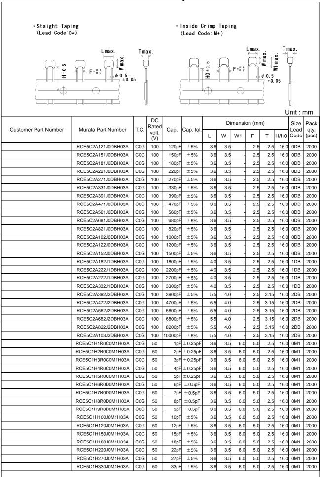
Inside Crimp Taping (Lead Code: M\*)
