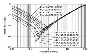
Common Mode Insertion Loss (Typ.)
