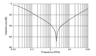
Differential Mode Insertion Loss (Typ.)
