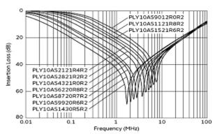
Differential Mode Insertion Loss-Frequency Characteristics
