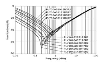
Common Mode Insertion Loss (Typ.)
