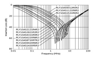
Differential Mode Insertion Loss (Typ.)
