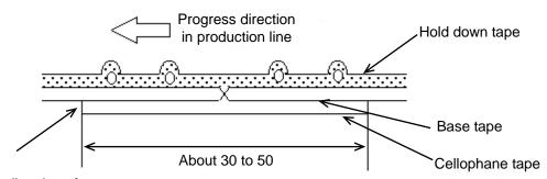
No lifting for the direction of progressing
