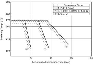
Perform soldering within tolerance range (shaded portion).
