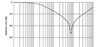
Common Mode Insertion Loss-Frequency Characteristics
