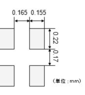
Accordingly increasing the solder volume, the mechanical stress to product is also increased. Excessive solder volume may cause the failure of mechanical or electrical performance.
