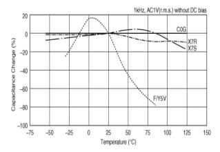
Capacitance - temperature characteristics
