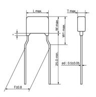
Coating extension does not exceed the end of the lead bend.
