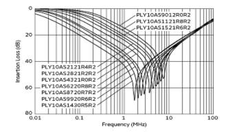
Differential Mode Insertion Loss (Typ.)
