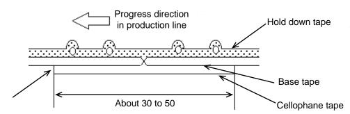
No lifting for the direction of progressing
