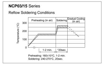
\* In case of repeated soldering, the accumulated soldering time should be within the range shown above figure 2.
