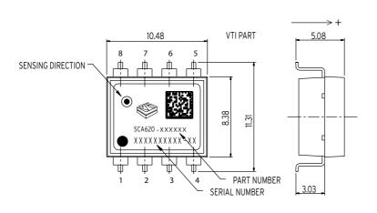
Acceleration in the direction of the arrow will increase the output voltage.
