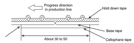
No lifting for the direction of progressing
