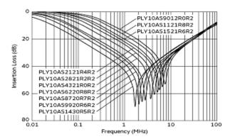
Differential Mode Insertion Loss (Typ.)
