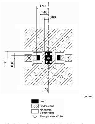
$^{\star}$  Line width to be designed to match 75 ohm characteristic impedance,  ${\rm Depending\ on\ PCB\ material\ and\ thickness}.$
