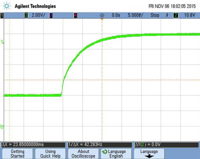
Start-up into a Pre-bias Load@25°C
