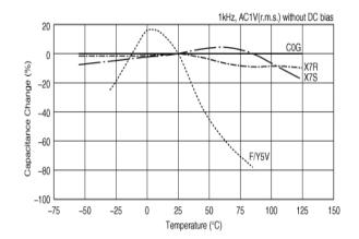
Capacitance - temperature characteristics
