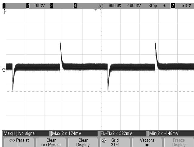
Step Load Transient Response (Vin=48V, Vout=nominal, Load=0, Iout=50 to 75 to 50% of full load, Ta=+25°C.) Trace 1=Vout, 100 mV/div., 2 mS/div.
