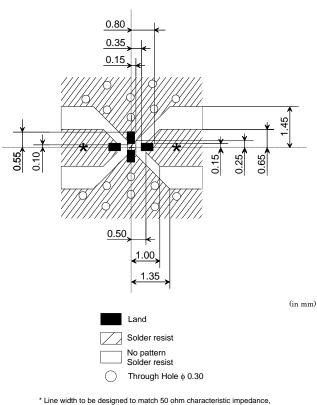
\* Line width to be designed to match 50 ohm characteristic impedance Depending on PCB material and thickness.
