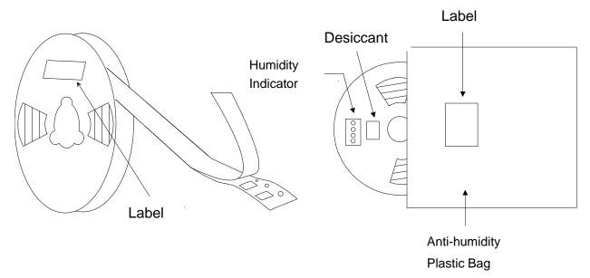
Tape and reel must be sealed with the anti-humidity plastic bag. The bag contains the desiccant and the humidity inductor.
