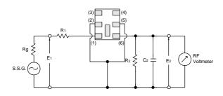
$$\begin{split} Rg &= 50\Omega \quad R1 = 280\Omega \pm 5\% \quad Rz = 330\Omega \pm 5\% \\ Cz &= 10 \pm 2 \, p\Gamma \; \text{(Including stray capacitance and Input capacitance of RF Volt Meter)} \\ E_1: S.S.G. \; \text{Output Voltage} \end{split}$$
