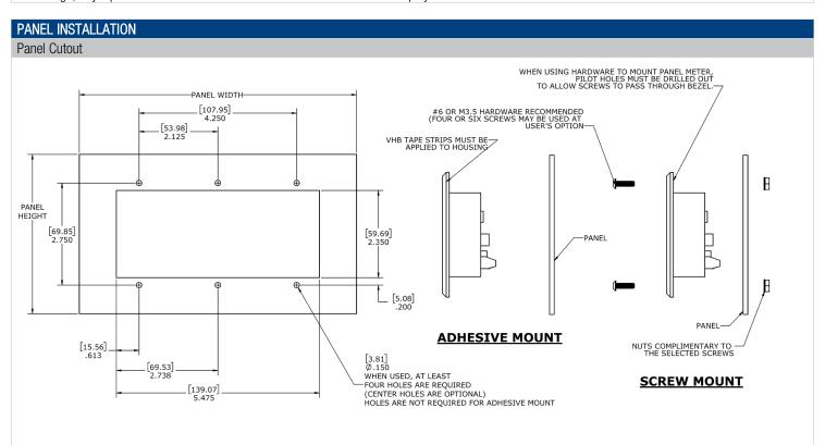
Note: When mounting panel meter with hardware, a four hole pattern (four outermost holes) or the six hole pattern may be used at the customer's option.
