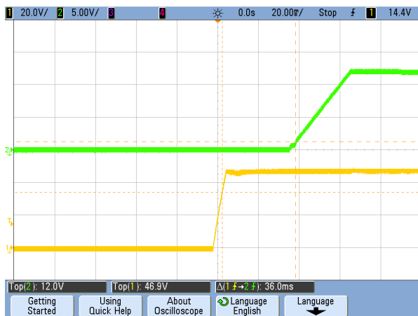
Figure 20. Vin Start-up Delay (CH2: Vout, CH1: Vin) (Vin=48V, Iload=0A, Cload=5500µF, Ta=+25°C, 20mS/div)
